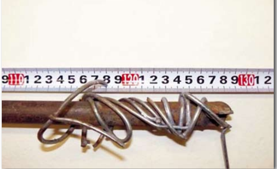
The drill steel, drill bit and entangled rib mesh
