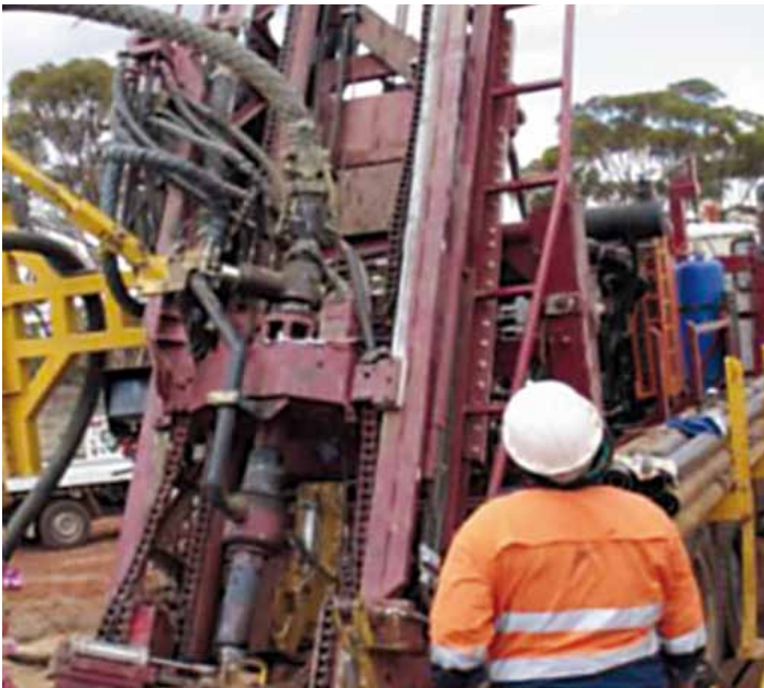
Mast with drill head and chains where they have come to rest
